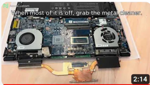
NV41 Series: How to replace the thermal paste.
