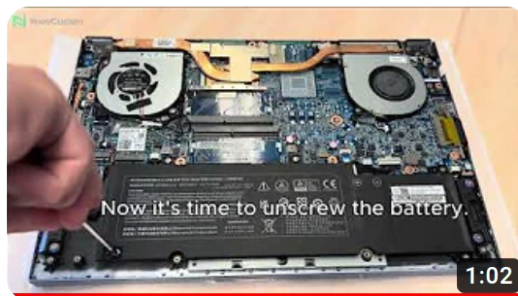
NV41 Series: How to replace the battery
